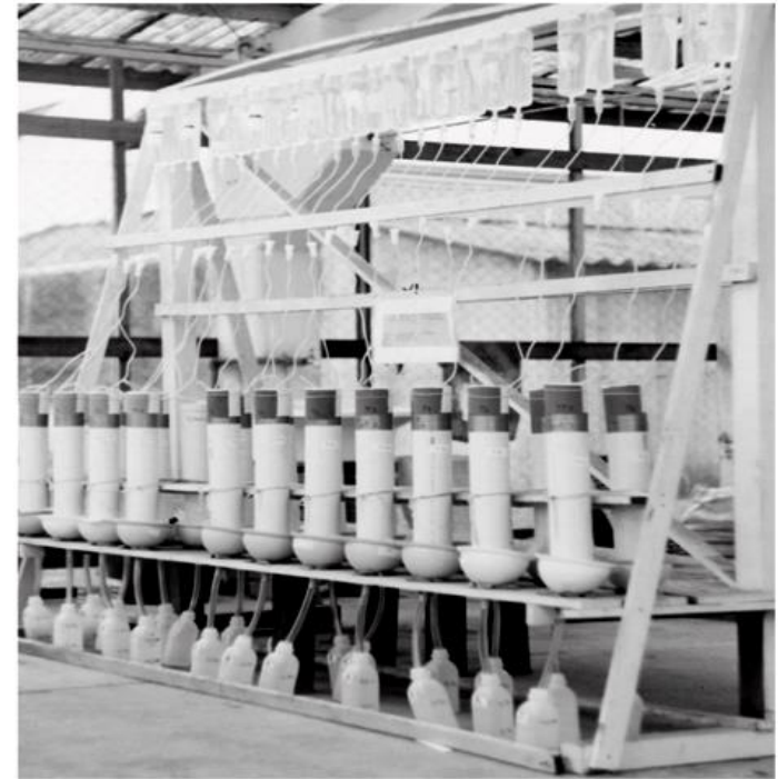
Figure 1 - Leaching columns experiment aspects
